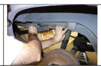
Mark a line on the Frame Rail at the front edge of the frame rail notch template. This will be the front of the frame rail cut. Measure 12 inches back from the back side of the frame rail notch template and make a line on the frame rail. This will be the rear of the frame rail cut.
